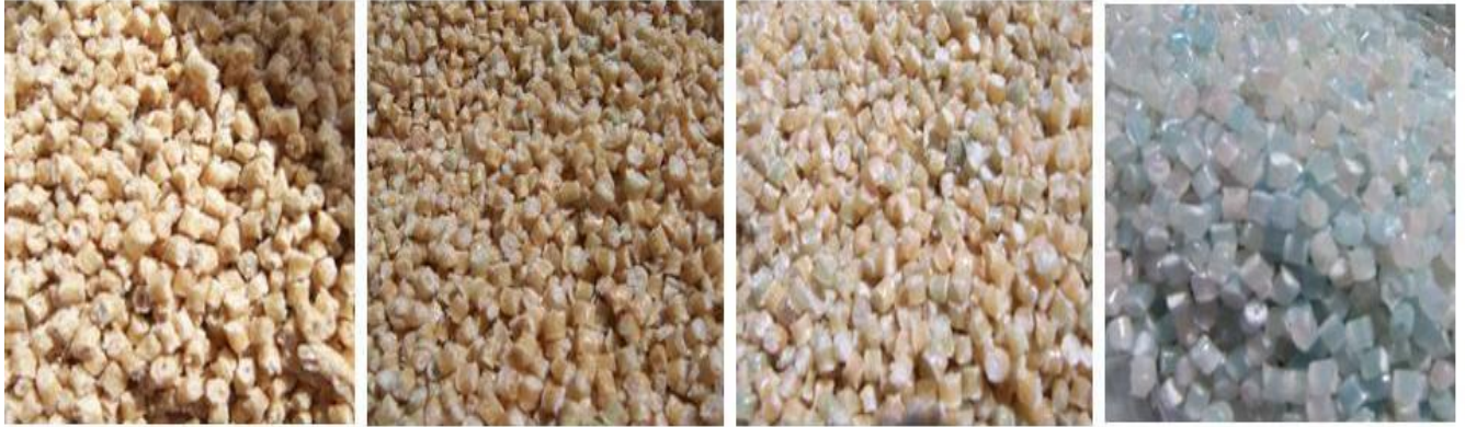
Figure 2: Pellets of wood-plastic composite in 30%, 20%, 10% and 100% PP FM, respectively.
