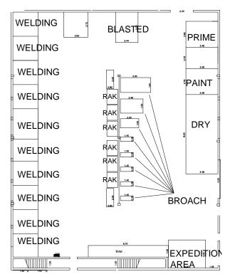
Picture 1 – Functional layout example in a metalworking industry Font: Silva (2009)
