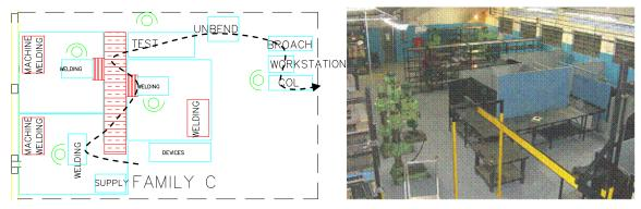
Picture 2 – Cellular layout example in a metalworking industry Font: (Silva, 2009)
